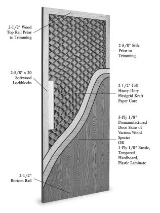
**RAILS:** 2-1/2" wood rails are standard. 15" maximum top and/or bottom rail. Hardwood rails by special request. All dimensions prior to factory trimming and prefitting.
